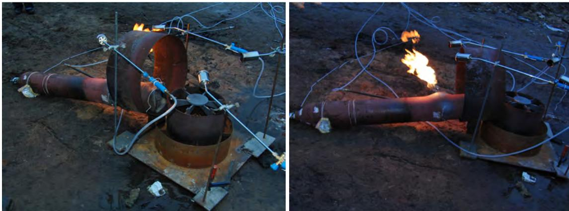
Figure 12: Broken gas cylinder after test 2
