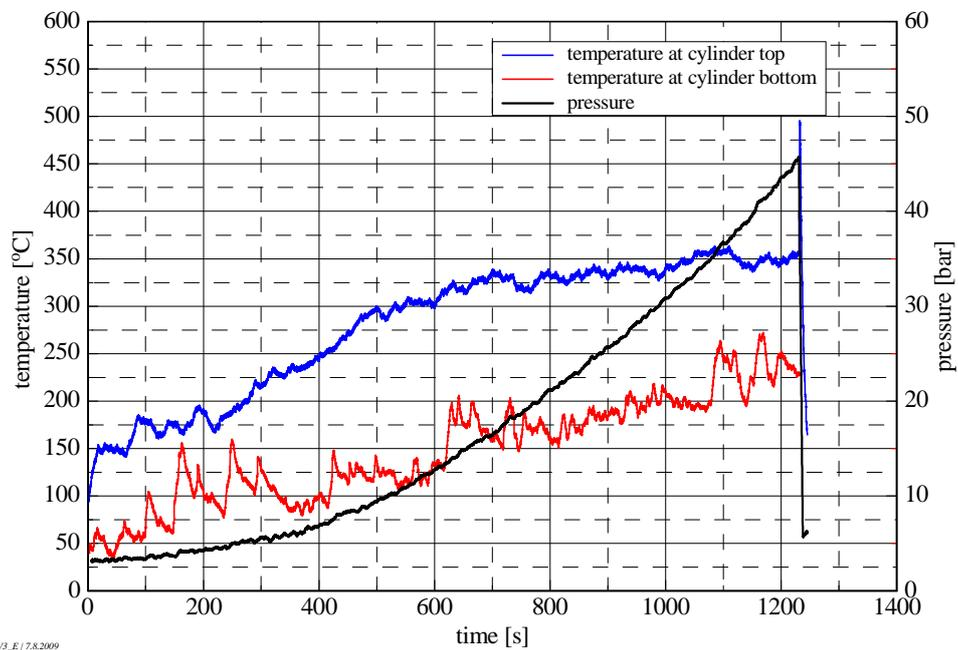
Figure 16: Wall temperature and pressure curves during the fire test with burners of an empty acetylene cylinder set in the horizontal position
