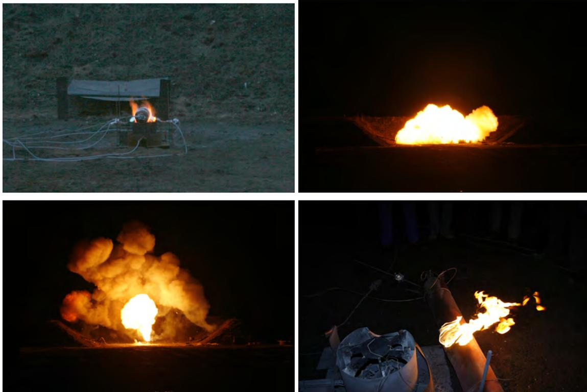
Figure 15: Image sequence of the fire test with burners of an empty gas cylinder set in the horizontal position (the left picture in the first row is retouched)
