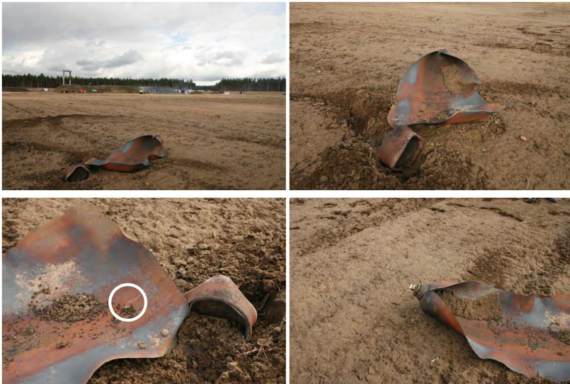
Figure 21: Burst acetylene cylinder after test 5
