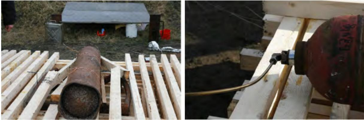
Figure 6: Set-up of the thermocouples for the temperature measurement in the cylinder inside (left picture) and detail of the modified gas cylinder valve for the pressure measurements (right picture)
