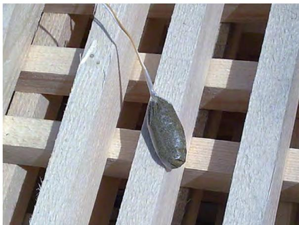
Figure 3: Detonation cap for the ignition of the wood pile
