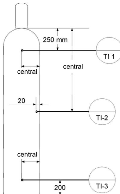
Figure 5: Location of the thermocouples for the measurement of the temperature inside a gas cylinder
