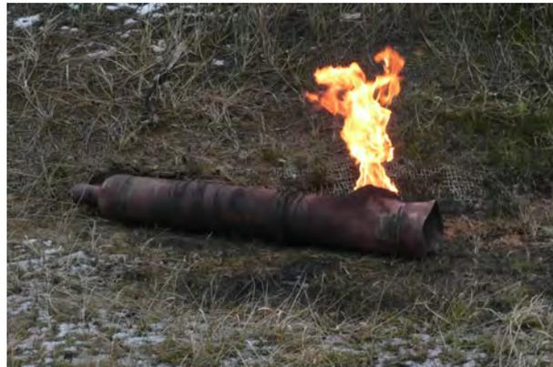
Figure 8: Burning solvent leaking from the cylinder after test 1
