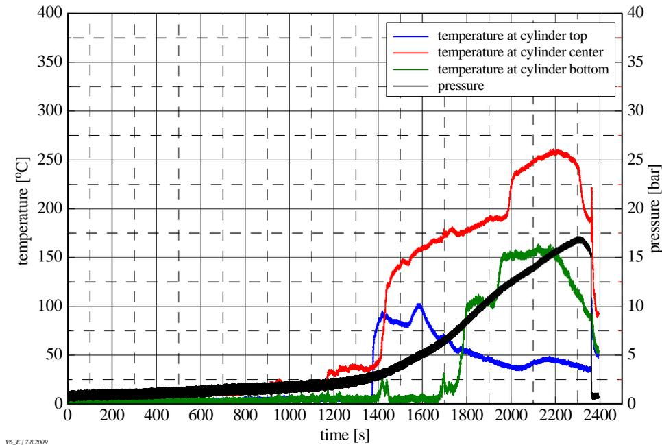
Figure 23: Temperatures in the porous material and pressure for an empty, horizontally orientated, acetylene cylinder exposed to a bonfire
