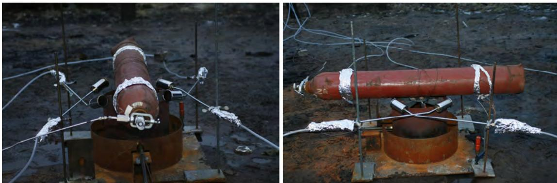
Figure 14: Set-up of the fire test with burners of an empty acetylene cylinder in the horizontal position.
