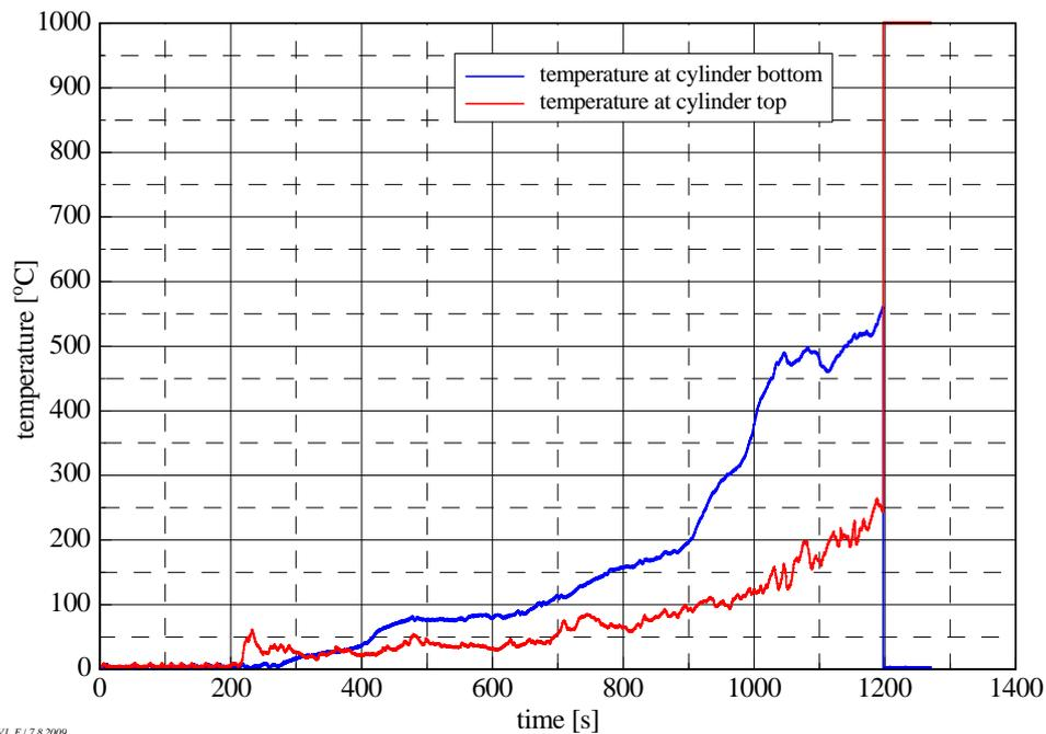
Figure 9: Wall temperatures over time for a full acetylene cylinder exposed to a bonfire in the standing position
