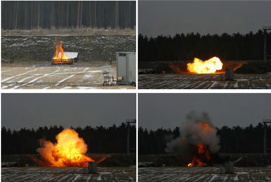
Figure 7: Image sequence of the exposure to a bonfire of a full acetylene cylinder in the standing position
