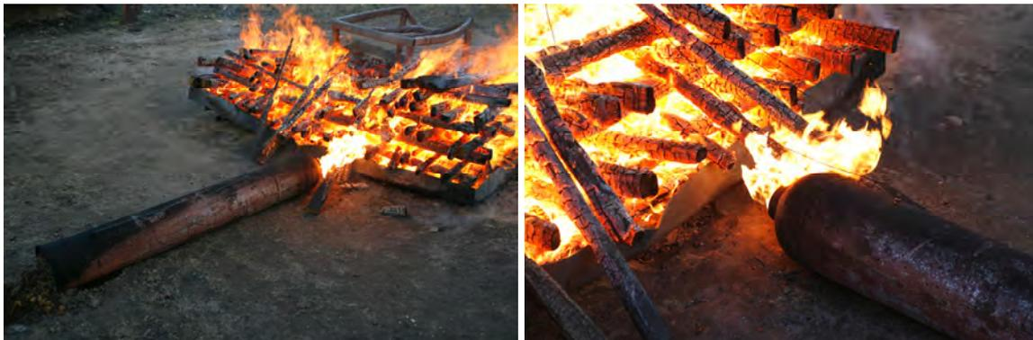
Figure 24: Image sequence of a bonfire test with an empty acetylene cylinder (horizontally orientated)
