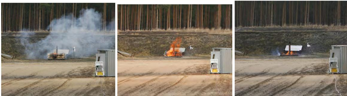
Figure 17: Image sequence of a bonfire test with an empty acetylene cylinder (vertically orientated)
