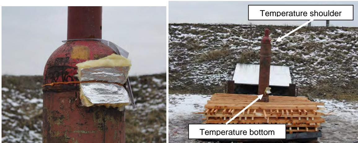
Figure 4: Fixing of the thermocouples for the temperature measurements on the cylinder wall
