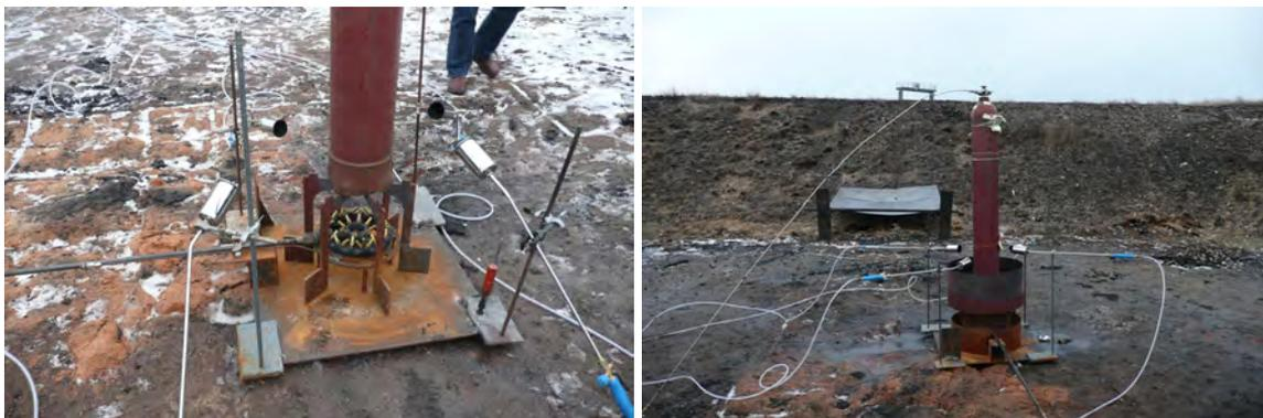
Figure 10: Preparation of the installation for the exposure to fire by means of burners of an empty acetylene cylinder in the standing position
