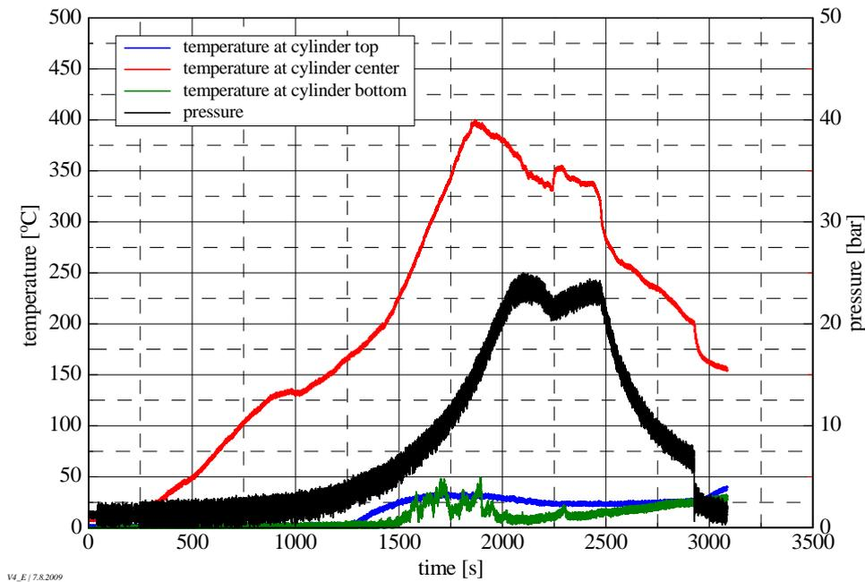
Figure 18: Temperatures in the porous material and pressure for an empty acetylene cylinder standing in a bonfire
