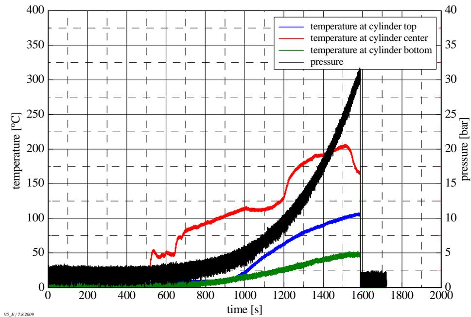
Figure 20: Temperatures in the porous material and pressure for an empty, horizontally orientated, acetylene exposed to a bonfire
