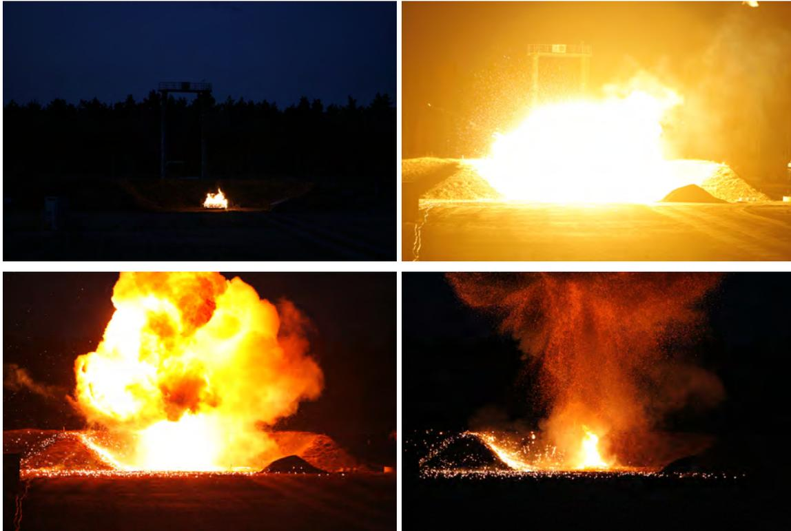
Figure 25: Image sequence of a bonfire test with a fully charged acetylene cylinder (horizontally orientated)
