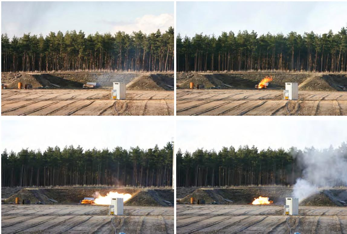
Figure 22: Image sequence of a bonfire test with an empty acetylene cylinder (horizontally orientated)
