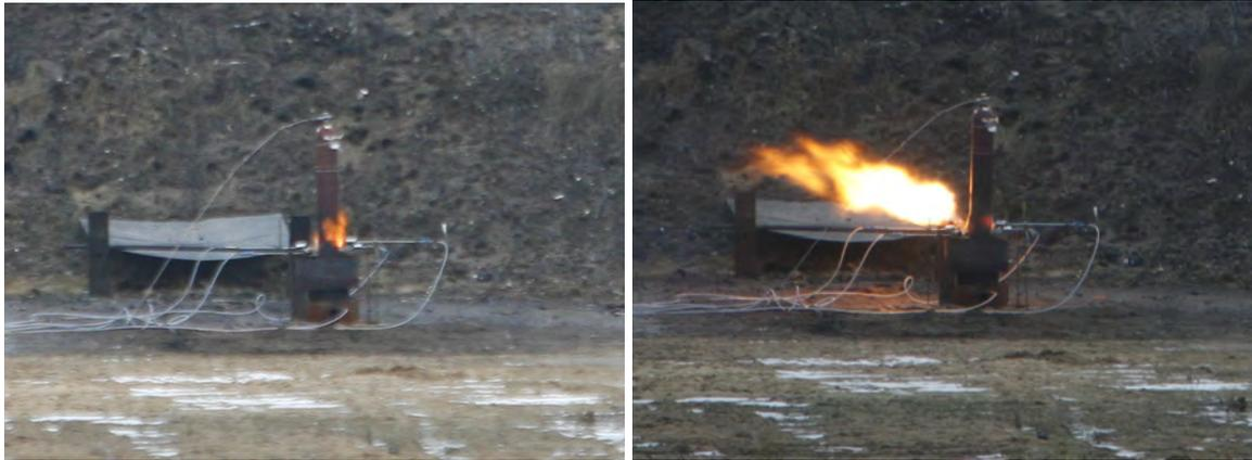
Figure 11: Test 2: gas cylinder with glowing walls during the exposure to fire (left picture) and detail of its later breaking (right picture)
