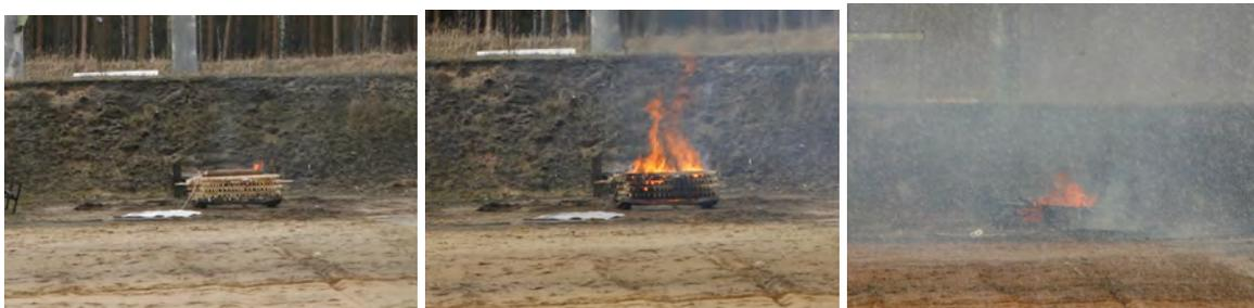
Figure 19: Image sequence of a bonfire test with an empty acetylene cylinder (horizontally orientated)
