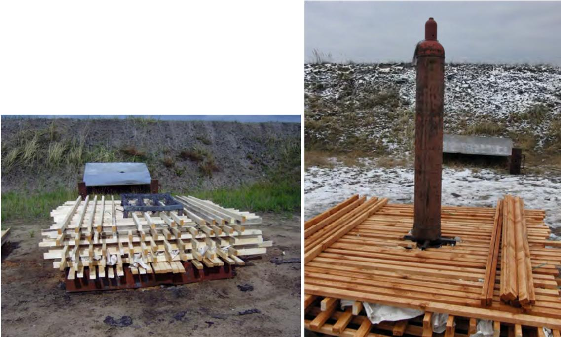
Figure 2: Supports in the wood crib pile for the exposition to fire of cylinders placed horizontally (left picture) and vertically (right picture)
