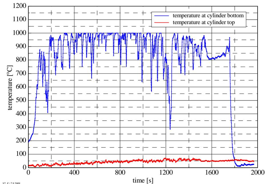
Figure 13: Wall temperatures over time for an empty gas cylinder in the standing position during the exposure to fire by means of a system of burners
